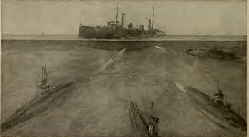
SUBMARINES ATTACKING A WARSHIP WITH DUMMY-HEADED TORPEDOES
